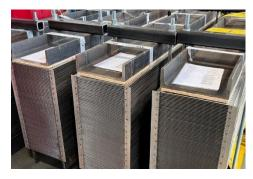
Similarly, the retrofit of an evaporator in a sugar factory in Baden-Württemberg is to be carried out at the beginning of next year. For this purpose, the existing Robert evaporator will be replaced by a much more efficient Hybrid Tubular falling film plate evaporator. The fully welded plate packs will have a heating surface of 4,400 m² and are already in production.
