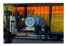
A global specialty chemicals company based in North Rhine-Westphalia needed a replacement condenser for an oxo plant. Since our hybrid could be integrated very well into the existing infrastructure and the low pressure losses required by the customer could be realized with it, we received the order. The recently delivered vacuum condenser weighs about 3.5 tons and offers an output of 867 kW on a heating surface of 163 m². Vapors and water are fed in counterflow.
